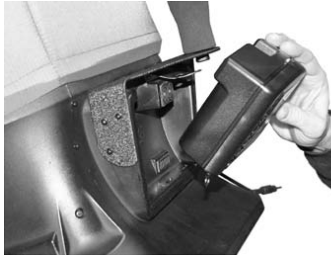
Figure 4 Attaching the Meter to the Capture Hood Base
