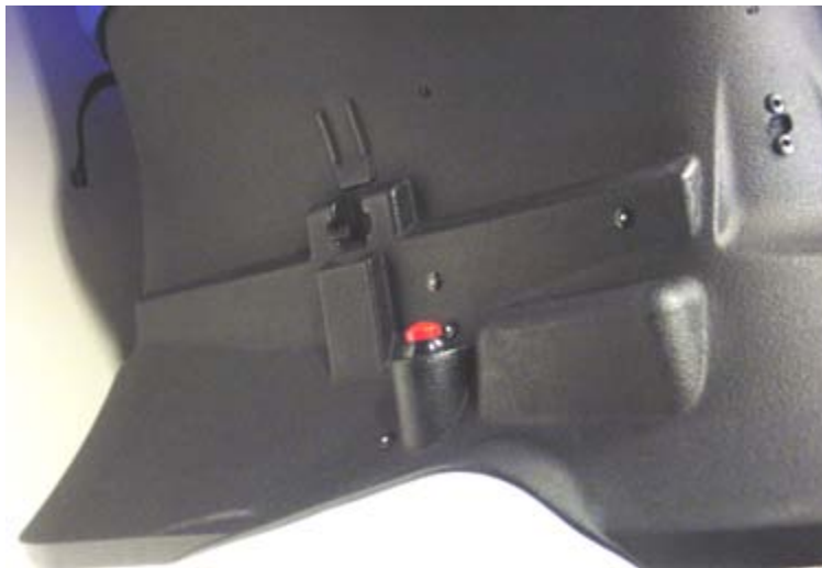
Figure 8 Red Hold Switch Location
