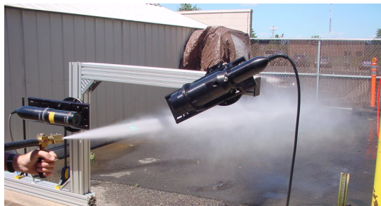
Figure 2: UHPS fire suppression spray (water) being measured by a TSI PDPA system
