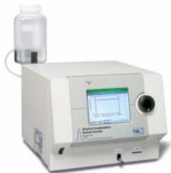
TSI Model 3776 Ultrafine Condensation Particle Counter (UCPC). Successor to the 3025A UCPC.
